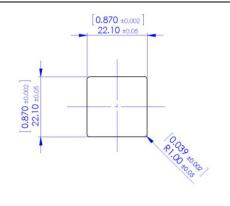
Panel thickness with standard nut: 1.00mm [0.039"] Minimum – 1.50mm [0.059"] Maximum
