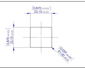
Panel thickness with standard nut: 1.20mm [0.047"] Minimum – 1.90mm [0.075"] Maximum
