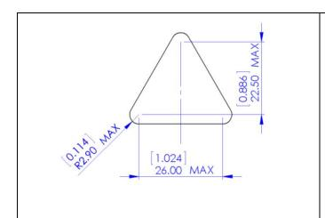
Insert Material – Acetate sheet or similar. Insert Thickness - 0.2mm [0.008"] Minimum -0.25mm [0.010"] Maximum
