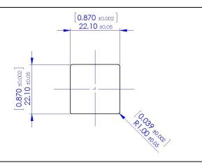
Panel thickness with standard nut: 1.20mm [0.047"] Minimum – 2.00mm [0.079"] Maximum
