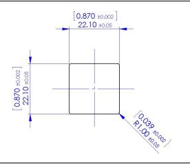
Panel thickness with standard nut: 1.20mm [0.047"] Minimum – 2.00mm [0.079"] Maximum
