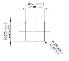
Panel thickness with standard nut: 1.20mm [0.047"] Minimum – 1.90mm [0.075"] Maximum
