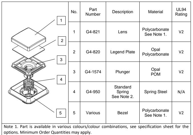
Note 2. All push buttons are supplied as standard with a light spring. A heavy force spring is available on request.
